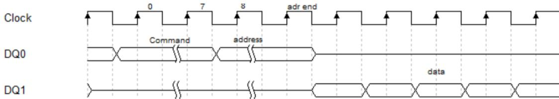
图 21-7 快速读指令 I/O Fast Read =0; MULTI COMM =0; SPI\_MODE=2'b00
