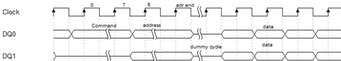
图 21-12 双路 I/O 快速读指令 I/O Fast Read = 1; MULTI COMM = 0; SPI\_MODE = 2'b01
